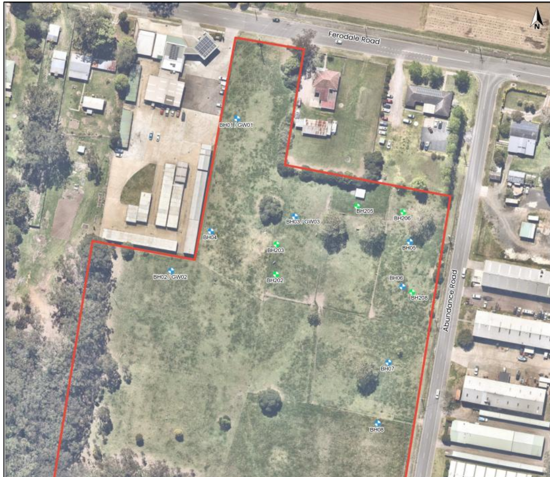
Figure 1: Survey Plan with Boreholes Indicated (Base Map Source: Nearmap)
